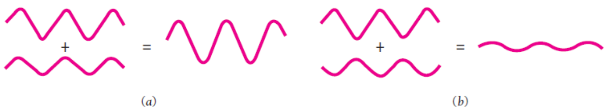
Figure 2.3 (a) In constructive interference, superposed waves in phase reinforce each other. (b) In destructive interference, waves out of phase partially or completely cancel each other.
