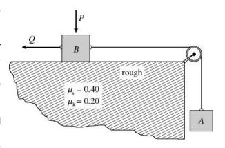
*P* equals 60 N. What is the maximum value of force Q, for which the system remains at rest? (In your solution, you must draw the free body diagrams.)
