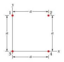
The particles have charges  $q_1 = -q_2 = 100 \ nC$  and  $q_3 = -q_4 = 200 \ nC$ , and distance  $a = 5.0 \ cm$ . What are the x and y components of the net electrostatic force on particle 3?
