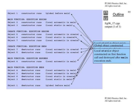
Figure 13: Order in which constructors and destructors are called. (part 2 of 2)
