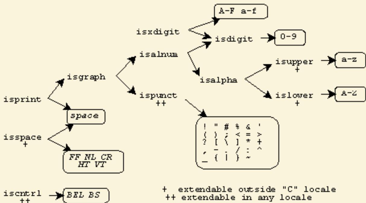
The diagram tells you that the function `isprint` returns nonzero for `space` or for any character for which the function `isgraph` returns nonzero. The function `isgraph`, in turn, returns nonzero for any character for which either the function `isalnum` or the function `ispunct` returns nonzero. The function `isdigit`, on the other hand, returns nonzero only for the digits 0–9.
