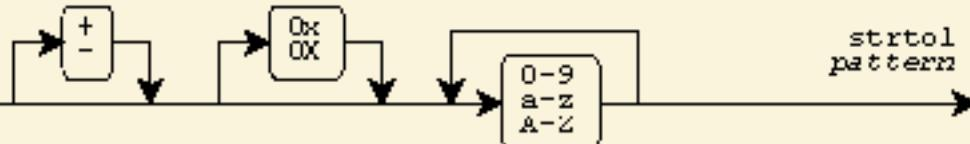
The function accepts the sequences 0x or 0X only when *base* equals zero or 16. The letters a-z or A-Z
