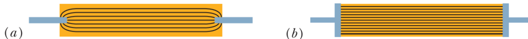
Fig. 26-8 Two ways of applying a potential difference to a conducting rod. The gray connectors are assumed to have negligible resistance. When they are arranged as in (a) in a small region at each rod end, the measured resistance is larger than when they are arranged as in (b) to cover the entire rod end.
