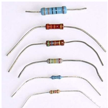
Fig. 26-7 An assortment of resistors. The circular bands are color-coding marks that identify the value of the resistance. (The Image Works)
